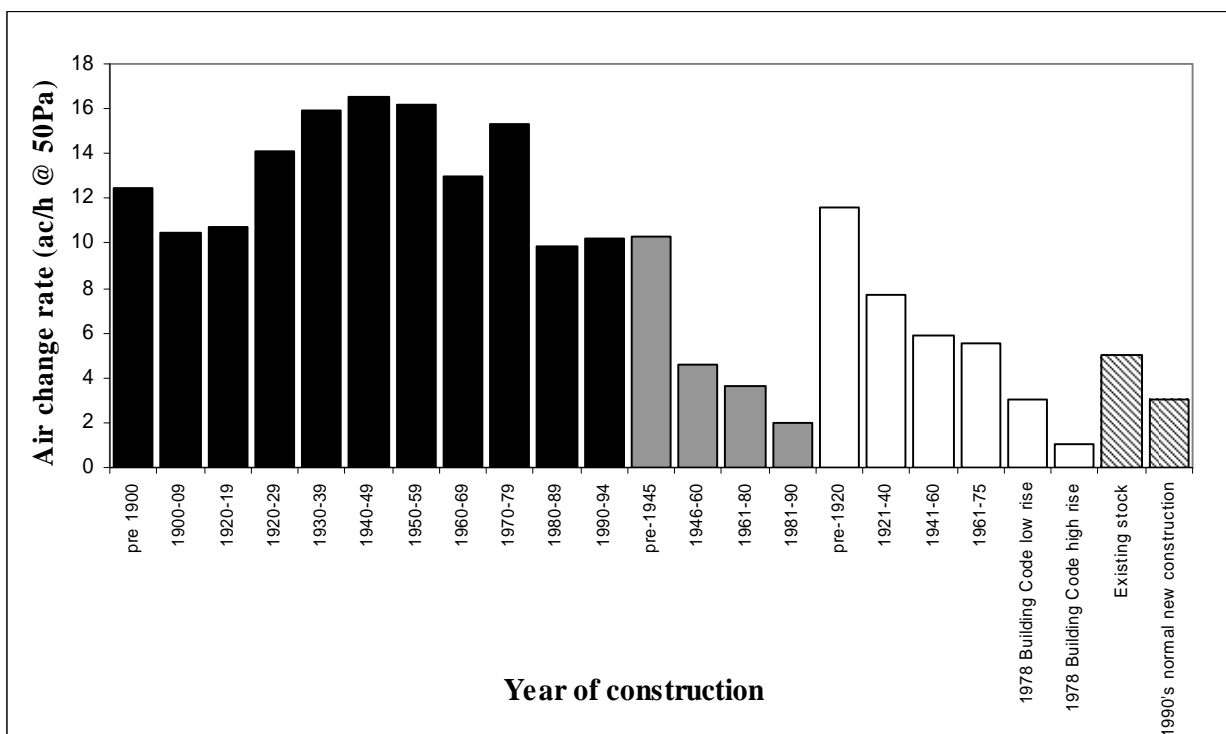
Figure 5 Effect of age on airtightness. Adapted from Stephen (2000) and Olivier (1999).
