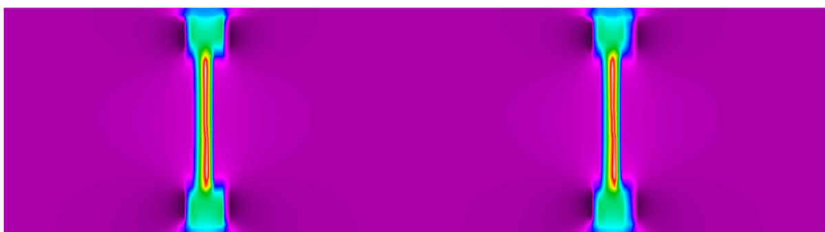
Figure 63 – Colour Flux Magnitude for Model I-beam Wall Panel
