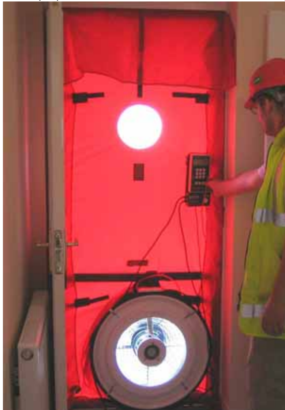
Figure 37 - Minneapolis Blower Door
