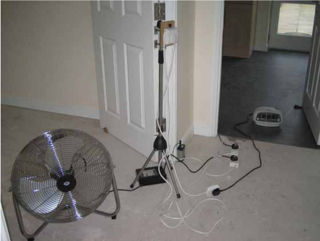
Figure 1 - Co-heating Equipment on Location in Test Dwelling at Stamford Brook
