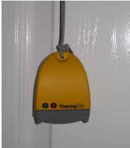
Figure 27 Tinytag Ultra Temperature Sensor
