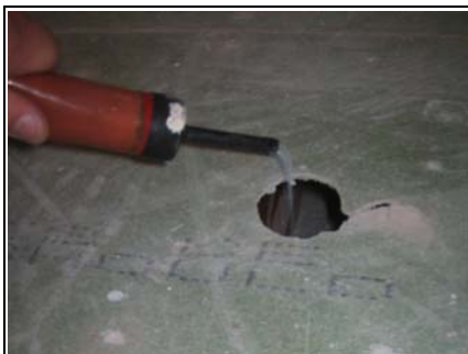
Figure 27. Air leakage directly into intermediate floor voids.
