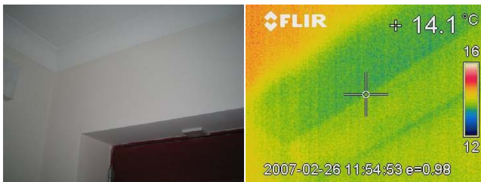
Figure 45. Stratification of temperature in the intermediate floor void directly above the recessed door detail (plot R110 - no induced pressure differential).
