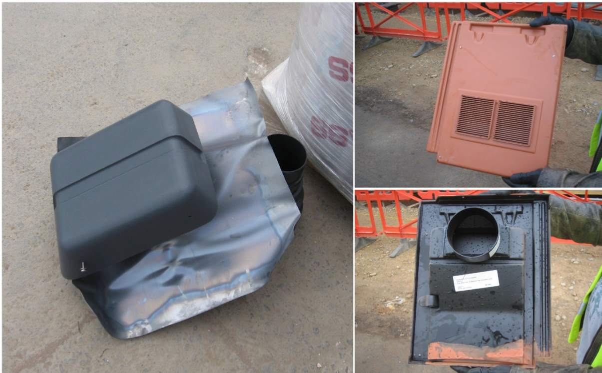
Figure 20 The replacement “mushroom-type” terminal vent, complete with lead slate fixing, and the originally-fitted “concealed” vent tile removed from the masonry prototype.
