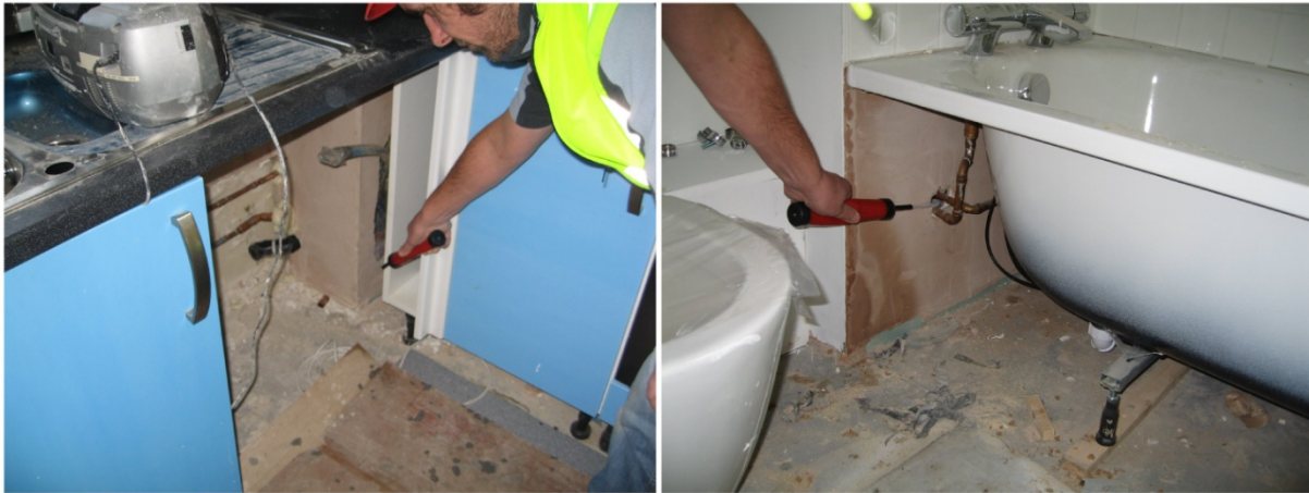
Figure 10 Air leakage into the service risers under dwelling pressurisation in the A1 prototype – 19/11/09.
