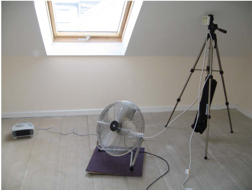
Figure 1 Coheating test equipment installed within a test dwelling.
