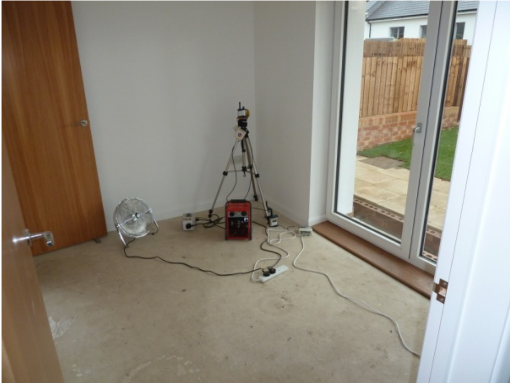
Figure 3 Main items of test equipment installed within a test dwelling.
