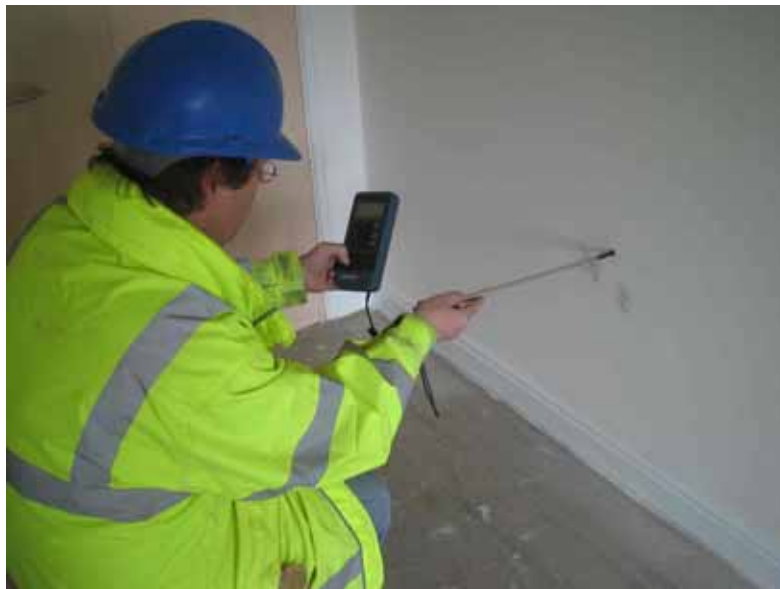
Figure 7 - Researcher Taking Cavity Air Flow Measurements through Hole in Party Wall
