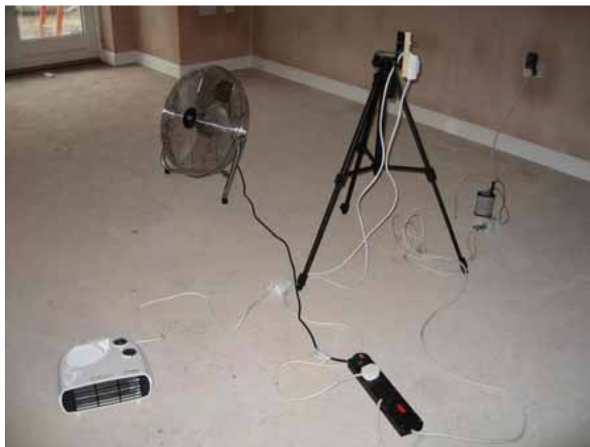
Figure A1 - Co-heating Equipment on Location in Room in Test Dwelling at Stamford Brook
