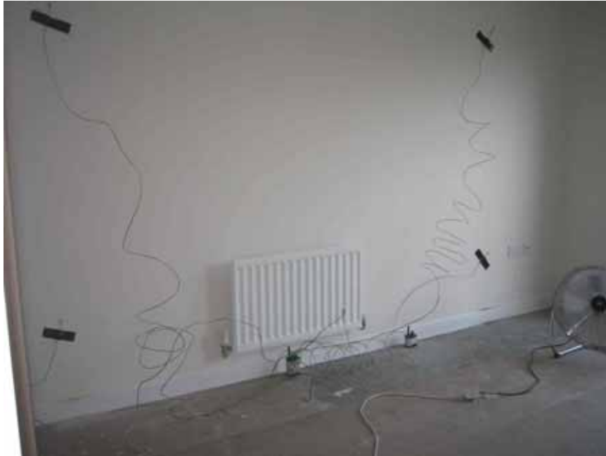
Figure 6 - Thermocouples in Position in Party Wall
