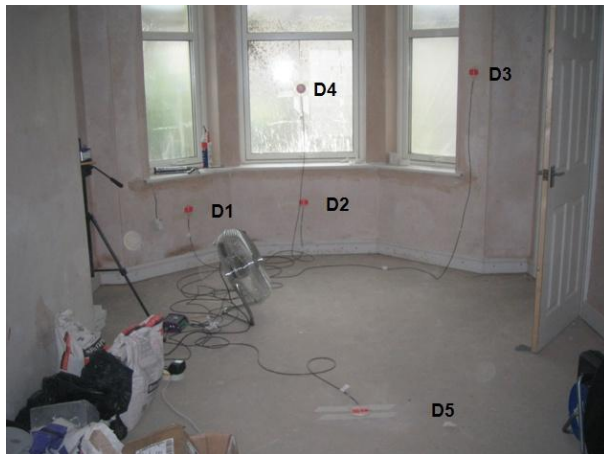
Figure 67 Phase 3 sensor locations and average U-values – Ground floor
