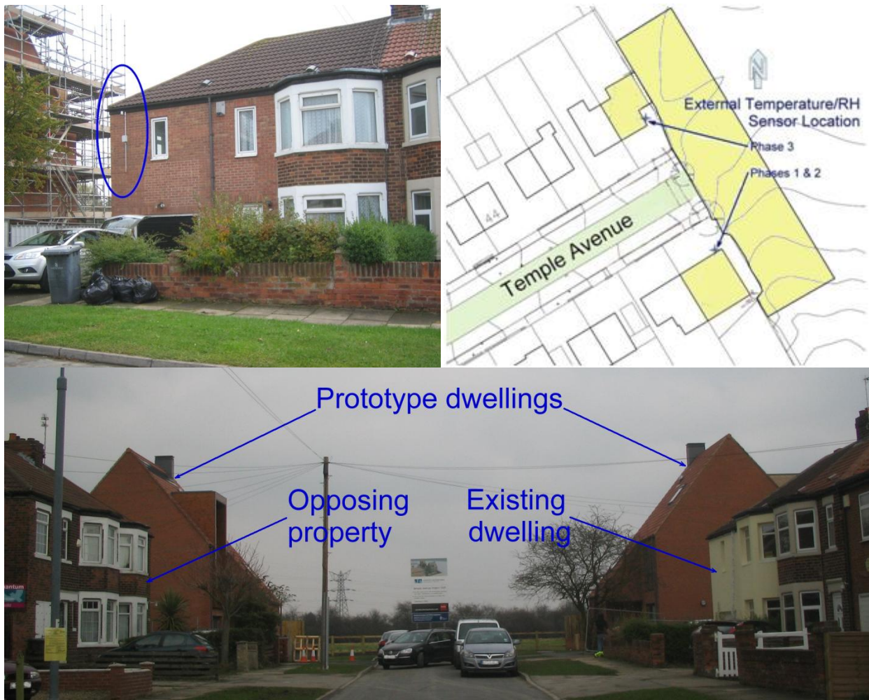
Figure 49 External temperature and relative humidity sensor was re-located from the front elevation of the test dwelling to the Gable wall of the opposing dwelling for the phase 3 coheating test.
