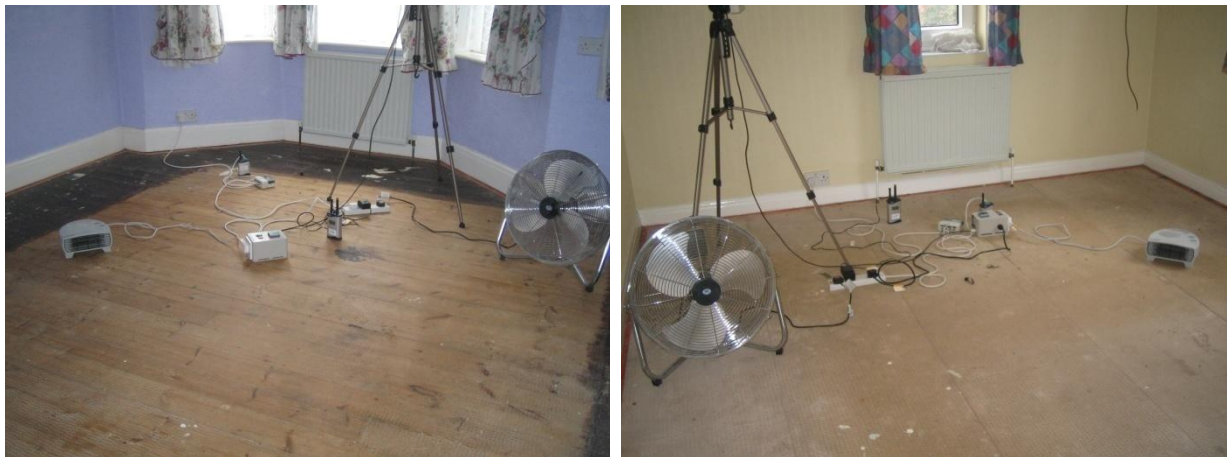
Figure 48 Coheating test equipment set-up in bedrooms 1 and 3.
