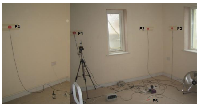
Figure 68 Phase 3 sensor locations and average U-values – 1 st floor
