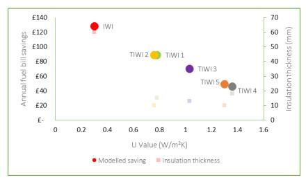
A dynamic simulation model (DSM) was used to evaluate the retrofits on a single case study home (assuming it is heated using a gas boiler) to identify annual fuel bill savings (the effects of TIWI 6 couldn't be modeled via DSM). As can be seen despite being only 20% to 30% the thickness of conventional IWI, and despite having U values between 0.8 and 1.4 when installed on solid brick walls, TIWI provides between 40% and 70% of the fuel bill savings that conventional IWI achieved.
