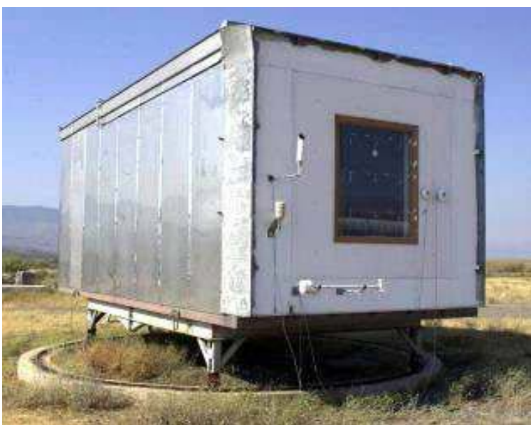
PASLINK test cell at LECE facility (CIEMAT, Spain)
